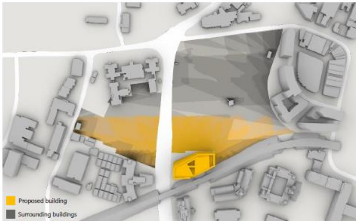
Figure 7—6 Transient overshadowing between 7.00 and 20.00 from the measured sunlight hours caused by the proposed and surrounding buildings at the 21 st of March
